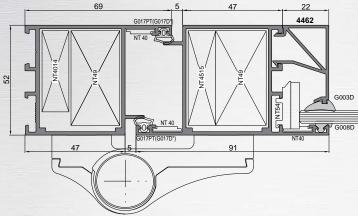
A non-insulated aluminium profile system designed for the manufacturing of internal constructions: glazed partitions, windows and doors.
